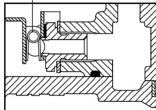
Fig. 2 Section of the main valve assembly - DN25 (1") only
