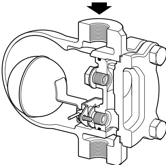
Fig. 1 CAS14 Screwed (vertical down)
