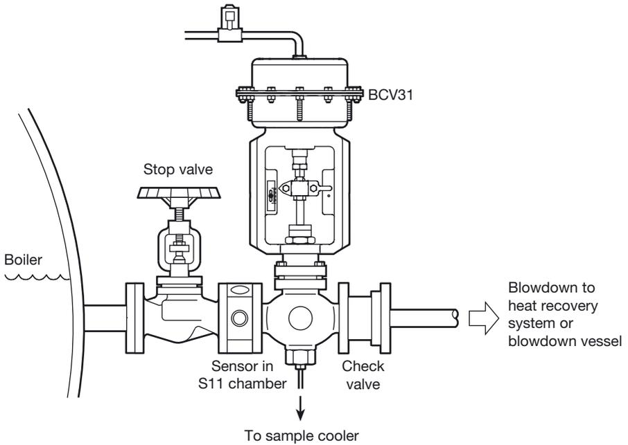
**Fig. 2 Installation on a boiler side connection**
