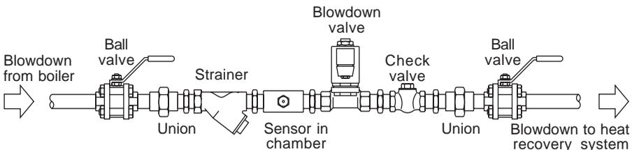
**Fig. 5 Typical installation**
