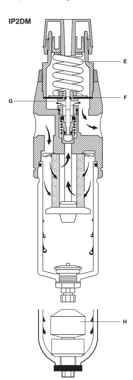
Metal bowl with sight level for IP2M, IP2AM and IP2DM
