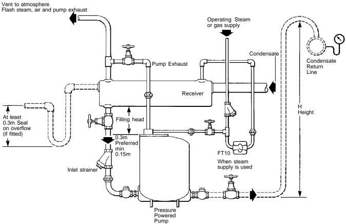
Recommended installation of pressure powered pump when fitted to a vented receiver. Flash steam must be vented or condensed ahead of pump inlet. Application details will dictate which of the following options will be necessary to accomplish this.
