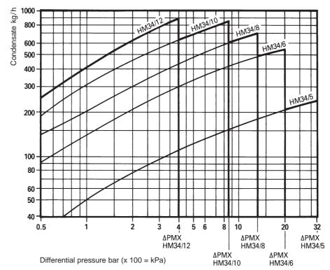
**Selection note:** Traps should be selected for the most appropriate working pressure differential and not on the basis of load, For example; DN25 HM34 with a load of 80 kg/h at 7 bar differential should be handled by an HM34/10 and not an HM34/5.
