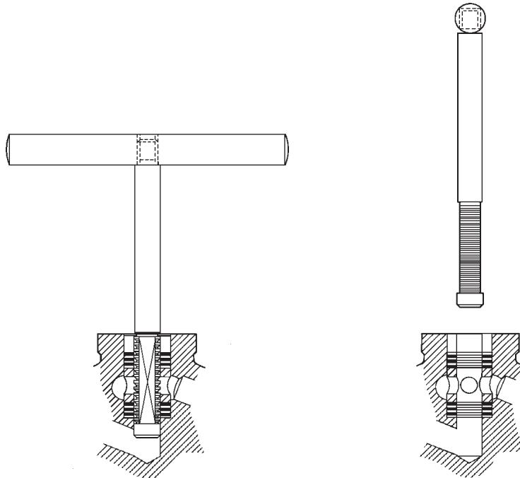
Fig. 4 View showing valve internals extractor tool
