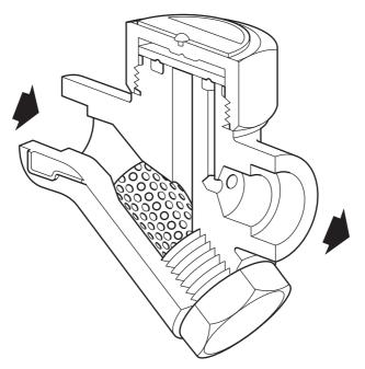
Fig. 1 TD42S2 thermodynamic steam trap
