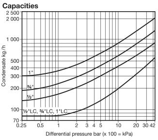
When sizing the TD42S2 it is important to ensure that the correct model is selected. This will ensure the required operation and maximum life. For mains drainage and tracing applications the LC version should be selected irrespective of pipe size.
