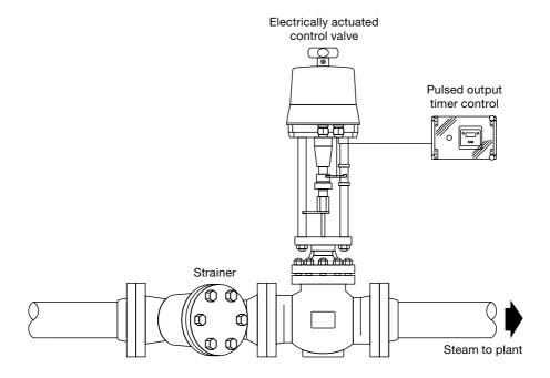
Fig. 1 Typical installation
