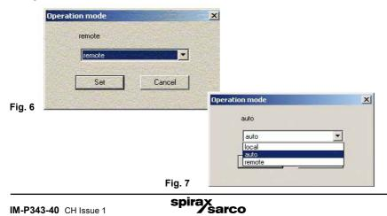
Choose the desired option and confirm by pressing the 'Set' button. The new value, see below, will appear highlighted in yellow. In order to send the new value to the positioner, press the 'Send' button at the top of the window as shown in the screen shot below.
