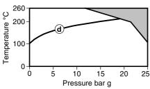
(d)-The steam saturation curve is added when relevant to enable users to easily find the specific operating points, e.g. 10 bar g saturated steam @ 185°C, 10 bar g steam with 20°C superheat or 10 bar g/250°C steam.
