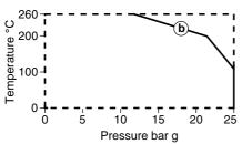
(b) - Is the maximum pressure which can be tolerated within the safety valve inlet tract. It is a function of the PN rating and and the body design/material.
