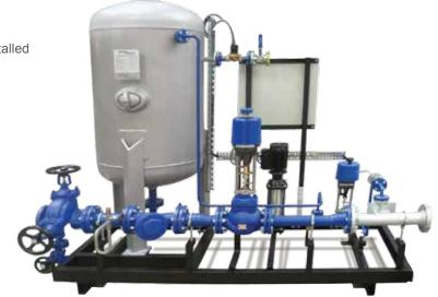
This desuperheater package was designed to reduce 13 bar g superheated steam at 275°C steam to 8 bar g at 5°C above saturation temperature. The customer uses superheated steam for its processes then uses the desuperheated steam to supply two Spirax Sarco heat exchangers for heating and hot water.
