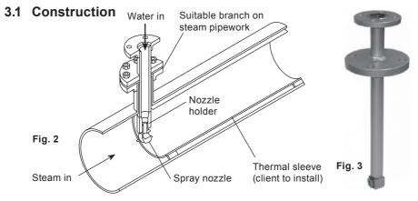
The spray nozzle desuperheater, type SND is an assembly which comprises one or more spray nozzles, cooling water inlet pipe, counter flange and cooling water inlet flange. The counter flange allows others to fit the SND onto a flanged branch in the steam pipework.
