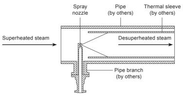
Fig. 4 SND spray nozzle desuperheater
