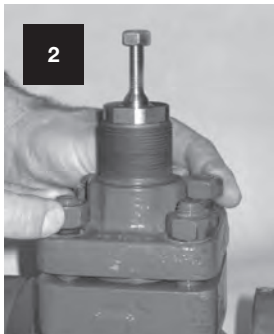
Finger tighten opposing bonnet nuts or bolts evenly in pairs.
