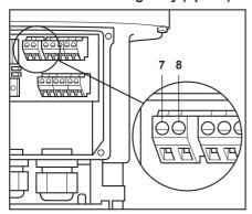
As an option, plugins 7 and 8 allows to display parameterisable fault indication to a control room. It is based on normally open contact relay. This option (ref. 6973) is linked with the communication software.
