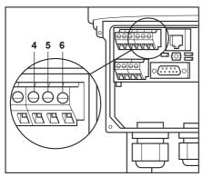
The AEL6 actuator could send as output an active position feedback, especially if a cut-off by position is requested.
