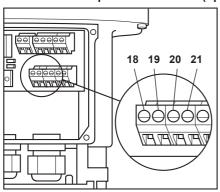
The activation points of the optionally available position switches are freely adjustable via cams. Plugging 18/19 and 20/21 provide potential free opening or closing contacts. The standard switches are rated to 230 Vac/5 A.
