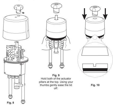
Note: When replacing the cover ensure that the two longest locating guides on the interior of the cover are aligned with the two recesses on the actuator housing. Firmly press down the actuator housing ensuring the 'O' ring on the actuator is completely concealed. For the AEL66\_ actuator remove the handwheel first by loosening the grub screw. Unscrew the 3 fixing screws around the bottom edge of the lid, then gently lift the lid off.
