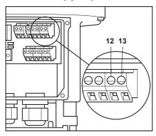
The AEL6 actuator could be fitted with a power safe fail package (ref . 6974 or 6975) which will power the actuator with a 24 V signal to ensure a safety position.
