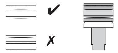
Fig. 3 Assembling the disc springs
