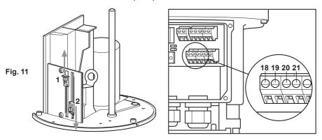
Section 3.5.6 shows how the switches are wired to the terminals. Fit the extend switch and the retract switch position (1) and (2) respectively in Figure 11.
