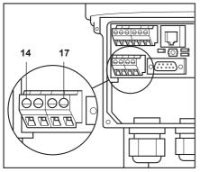
The AEL6 actuator could provide a 24 Vdc at maximum at 100 mA unregulated output voltage to an external process sensor.
