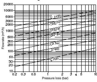
Pressure loss diagram with the valve open at 20°C. The values indicated are applicable to spring loaded valves with horizontal flow. With vertical flow, insignificant deviations occur only within the range of partial opening.
