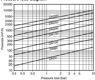
Pressure loss diagram with the valve open at 20°C. The values indicated are applicable to spring loaded valves with horizontal flow. With vertical flow, insignificant deviations occur only within the range of partial opening. The curves given in the chart are valid for water at 20°C. To determine
