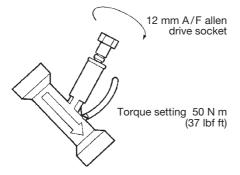
Fig. 2 Insert a 12 mm A/F hexagonal allen socket into the gun handle to a torque of 50 N m (37 lbf ft).
