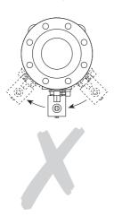
Fig. 2 Incorrect installation for liquid service
