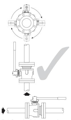
Fig. 3 Correct installation for gas service
