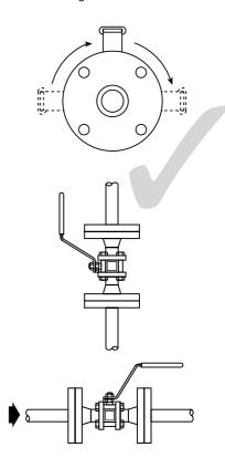
Fig. 3 Correct installation for gas service
