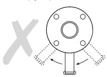
Fig. 2 Incorrect installation for liquid service
