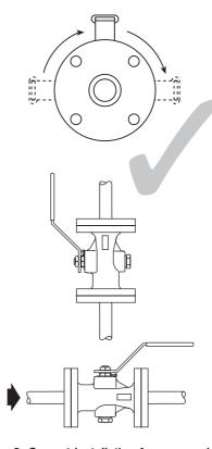
Fig. 3 Correct installation for gas service
