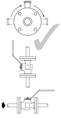
Fig. 3 Correct installation for gas service
